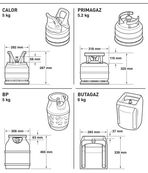
Maximum LPG cylinder capacity INSIDE cabinet is 6 kg. The length of hose must not exceed 1.5 metres.
