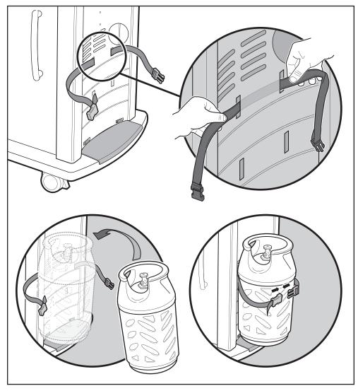
Maximum LPG cylinder capacity OUTSIDE cabinet is 13 kg. The length of hose must not exceed 1.5 metres.
